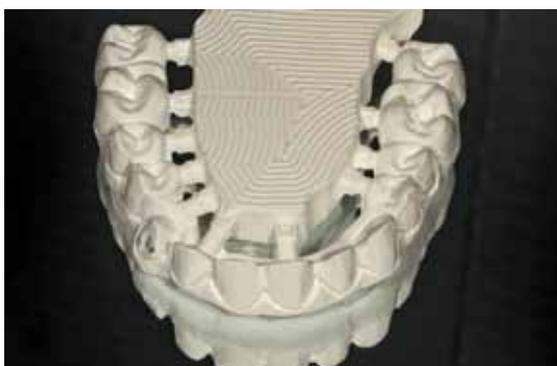
Fig. 8 Grinding upper restorations before sintering
