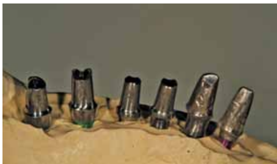
Fig. E Titanium implant abutments scanned using 3Shape digital scanner.
