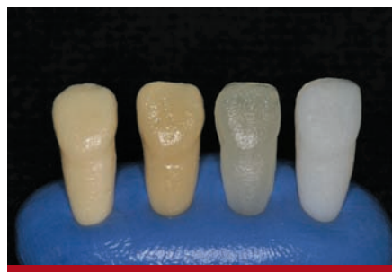
Figure 6 The technician tests the porcelain system by making and firing sample tabs in the laboratory. The sample tabs (left to right) are made of: opacious dentin, dentin, translucent, and enamel.
