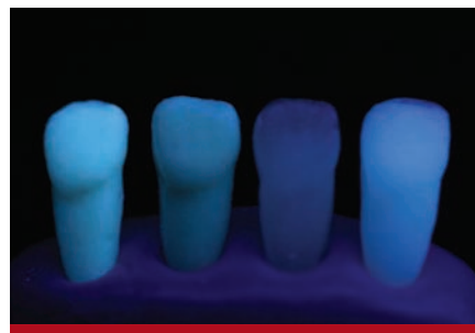
Figure 7 Under ultraviolet lighting, the sample tab's appearance should be checked for translucency.
