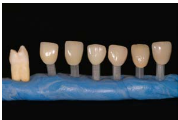
Figure 5: Appearance of a natural tooth, and various all-ceramic materials and metals with a variety of porcelains.
