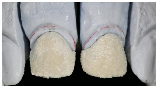
**Fig. A** Fluo crystals give an even masking of opaque to the metal coping.
