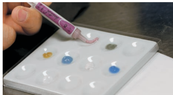
Fig. F Luster Pastes are dispensed from syringes and are thicker than glaze.
