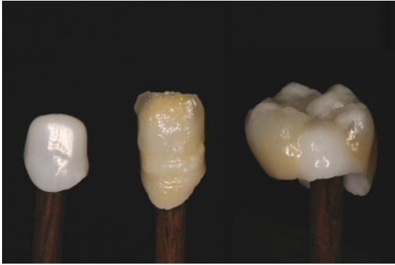
Figure 11: The zirconium coping is white; internal colors give the chroma shade and the finished restoration matches natural tooth. The molar distal lingual cusp has no porcelain on it, showing the white zirconium coping.
