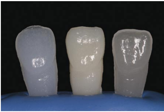
Figure 9: Laboratory porcelain sample test for the opal, enamel and transparency. The color is slightly different from the factory-made shade tab, because of variations in laboratory oven temperature.
