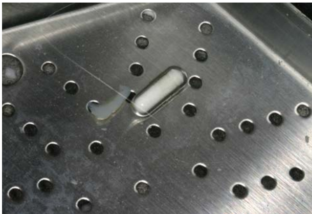
Fig. 25. Finally heat-cured under water (oxygen free) by adding oxygen scavenger in water.
